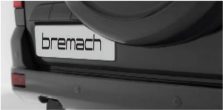
Rear parking sensors on the bumper and rear view camera in the tailgate handle
