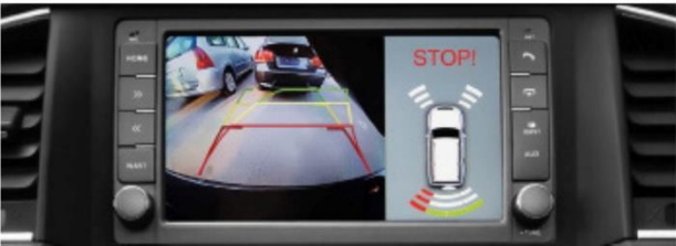
When backing up a vehicle, a color display shows the view from the rear camera with dynamic indexing lines and front and rear parking sensor signals
